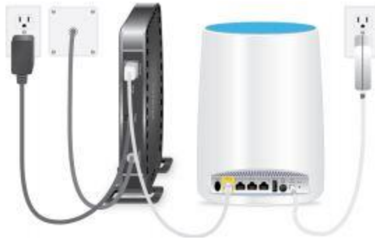
Figure 3 - Orbi Router Wiring
